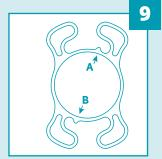
implanted, orientation features of the lens must be oriented at the top right (A) and at the bottom left (B).
